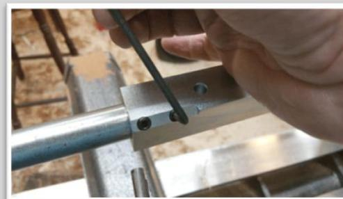
9. If there is not a cutting tip in the holder install it now. Move the tool rest under the tool holder bar and adjust upward until the tool tip is on center.
