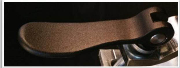
2. Hold the lower bolt head with your left index finger and hand tighten the nut with your right hand.
