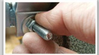
**3. Make sure the weld on the clamp block does not touch the quill.**
